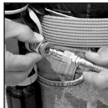
3) Disconnect the hose and pneumatic tool from the regulator.
