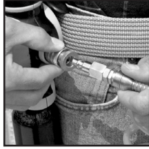
2) Connect hose to regulator fitting
