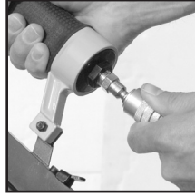
3) Connect hose to pneumatic tool
