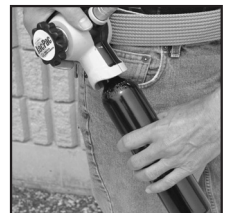
4) Unthread CO 2 cylinder from regulator. Store all components in the convenient storage case
