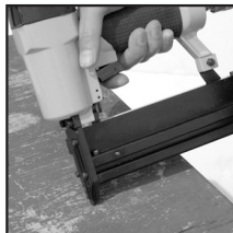
2) Discharge pneumatic tool several times to relieve the system of any remaining CO 2
